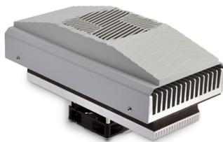
Thermoelectric units are solid state devices which operate as heat pumps to transfer heat using the Peltier effect. This cost-effective solution is ideal for the climate control of small enclosure. No compressor or moving part (except the fans), no hazardous gases and not sensitive to vibrations are the main advantages.
