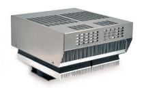
Thermoelectric units are solid state devices which operate as heat pumps to transfer heat using the Peltier effect. This cost-effective solution is ideal for the climate control of small enclosure. No compressor or moving part (except the fans), no hazardous gases and not sensitive to vibrations are the main advantages.
