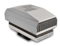
Thermoelectric units are solid state devices which operate as heat pumps to transfer heat using the Peltier effect. This cost-effective solution is ideal for the climate control of small enclosure. No compressor or moving part (except the fans), no hazardous gases and not sensitive to vibrations are the main advantages.
