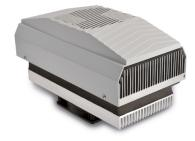
Thermoelectric units are solid state devices which operate as heat pumps to transfer heat using the Peltier effect. This cost-effective solution is ideal for the climate control of small enclosure. No compressor or moving part (except the fans), no hazardous gases and not sensitive to vibrations are the main advantages.
