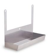
Drip tray is a stainless steel accessory to be positioned under the thermoelectric unit. It is used to collect the condensate generate on the cold heat sink inside the enclosure. Suitable for vertical installation.
