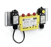
Flashing signal devices monitor the voltage status of electrical panels and carry out inspection and maintenance operations in total safety. They prevent accidents by warning the operator that the electrical system is active by means of flashing lights. By integrating with auxiliary contacts, such as limit switches or additional interlocks, it is possible to control the electrical voltage inside the cabinet when the door is opened.
