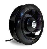
Radial fans with backwards-curved blades are used in suction, even without scroll, in high-speed applications. As a result of these characteristics, they can determine a high-pressure flow with reduced airflow. Radial backwards-curved fans have good air efficiency and a low noise level.
