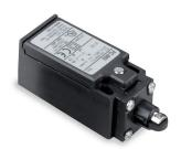
The limit switches ensure safety during maintenance work inside the electrical panels. They are applied on the frame of the cabinet and can turn on the lights, turn off a fan or a heater or cut off the power supply in general when the door is opened or closed.
