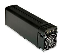
Fandis PTC heaters are used for warming up the air inside enclosure, protecting electrical and electronic components from condensation and corrosion. These H series PTC heaters with builtin fan ensure quick distribution of heat and are available in two versions: in metal or plastic, with low surface thermal conductivity to keep safe maintenance operations.
