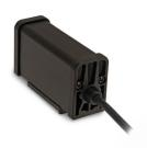
Fandis PTC heaters are used for warming up the air inside enclosure, protecting electrical and electronic components from condensation and corrosion. These H series PTC heaters with cable connection are available in two versions: in metal or plastic, with low surface thermal conductivity to keep safe maintenance operations.
