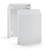
A protective cover for exhaust filters and filter fans in powder coated RAL 7035, UL Type 4. It safeguards the enclosure inside against rain, water jets and foreign particles, by increasing the protection class to IP56. Available also in stainless steel (AISI 304) and UL Type 4X version equipped with a FDA-compliant silicone gasket for a safe use in food industry or outdoors.
