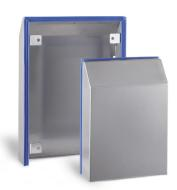
A protective cover for exhaust filters and filter fans in stainless steel (AISI 304) and UL Type 4X version equipped with a FDA-compliant silicone gasket for a safe use in food industry or outdoors. It effectively safeguards against rain, water jets and foreign particles by securely sealing the ventilation openings, by increasing the protection class to IP56. Available also in powder coated RAL 7035, UL Type 4.
