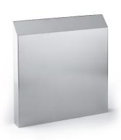
A protective cover for exhaust filters and filter fans in stainless steel (AISI 304) to safeguard against rain, water jets and foreign particles, by increasing the protection class to IP56. Available also in powder coated RAL 7035, UL Type 12 and in UL Type 4X version equipped with a FDA-compliant silicone gasket.
