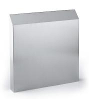
A protective cover for exhaust filters and filter fans in stainless steel (AISI 304) to safeguard against rain, water jets and foreign particles, by increasing the protection class to IP56. Available also in powder coated RAL 7035, UL Type 12 and in UL Type 4X version equipped with a FDA-compliant silicone gasket.
