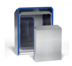
Stainless steel (AISI 304) cover with FDA-compliant gasket to be applied to exhaust filters and filter fans to protect the internal components of the electrical panel from water jets and the ingress of solid objects, in order to elevate the protection rating to IP56. Ideal for applications with high hygienic standards in the Food & Beverage sector and for outdoors. Also available in powder-coated steel cover RAL 7035.
