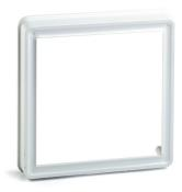
Adapter is a plastic frame that allows the filter fan to sit in a semi built-in position in the enclosure, reducing the internal depth. It is ideal when installation space within the enclosure is limited, because the adapter is screwed directly on the cabinet's external wall and the ventilation unit can be then simply clipped onto.
