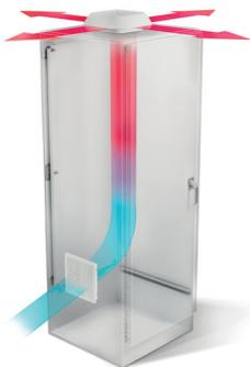
Hot air can also be expelled from the roof of the cabinet if, for instance, the sides of the cabinet are covered by obstacles, walls or by the sides of other cabinets. In a perfect configuration, an exhaust filter is positioned at the bottom of the cabinet. The lower pressure generated by the roof unit draws in cold air from outside through the exhaust filter to enhance internal air flow and the dissipation of heat.
