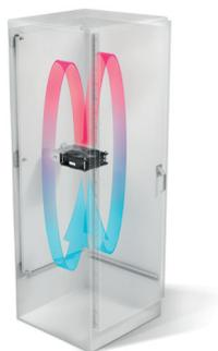
The use of a swivelling fan is an alternative solution for a better air circulation inside the electrical cabinet. This fan distributes heat to reduce the temperature, cools local hot spots and disperses cold air emitted by cooling units.
